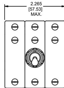
Panel Mounting Details: Tolerance  $\pm .005$  [.13] Unless noted.
