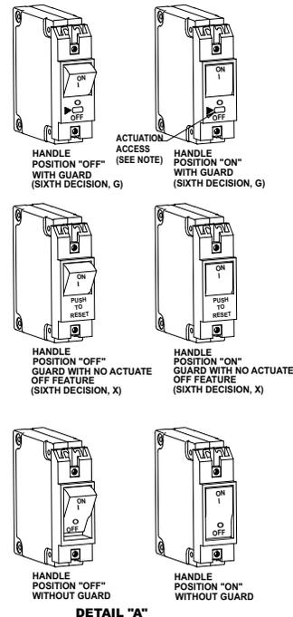
NOTE: ACCESS IS LIMITED TO A DEVICE SMALLER THAN THE UNDERWRITERS LABORATORY "ARTICULATED PROBE" DEFINED IN UL-489 FIG. 11.1.7.2.1.
