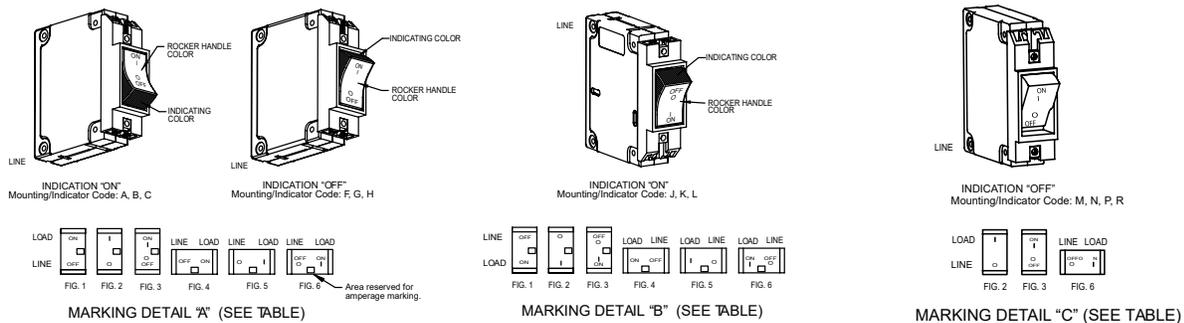
Notes: The LEL family of circuit breakers are designed to meet 8mm creepage and clearance requirements for installation Category 111, pollution degree 3, Case A as measured in IEC 664. Intended for use in equipment designed to comply with IEC 380, 435, 601.
