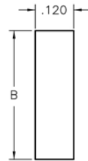
DETAIL A MAXIMUM CABLE OPENING SEE NOTE 4
