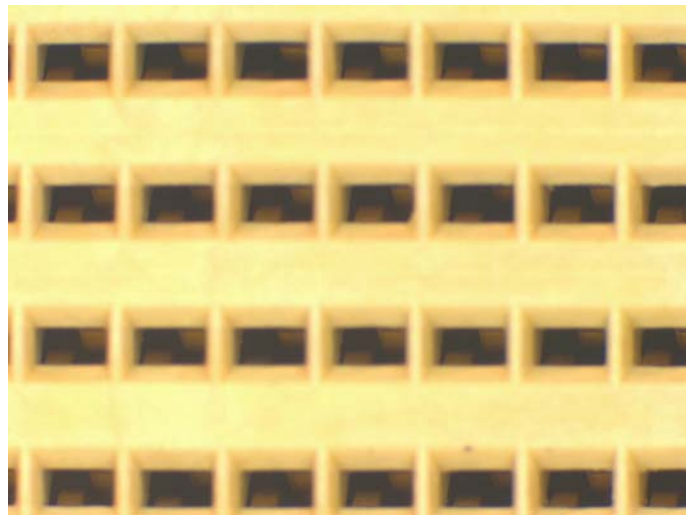
Fig. 2 – Mated VR After Salt Spray
