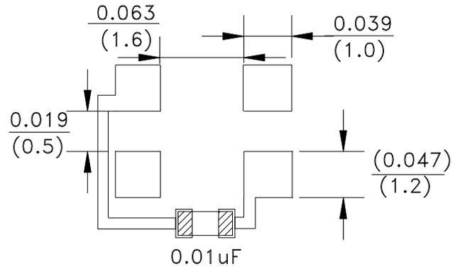
Note 1: It is not recommended that paths go underneath the oscillator. If needed, please use multi-layer PCB board or resist coating.
