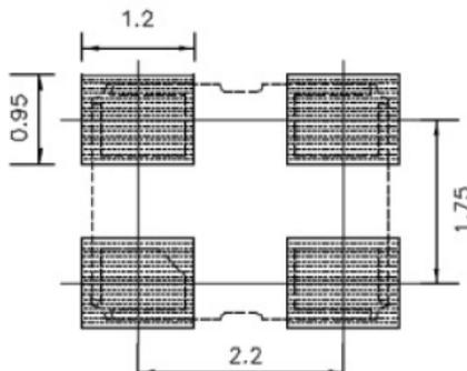
Note 1: It is not recommended that paths go underneath the oscillator. If needed, please use multi-layer PCB board or resist coating.
