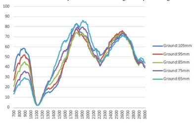
Reference efficiency data with different ground plane length:
