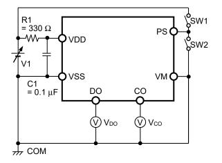
Figure 3 Test Circuit 1
