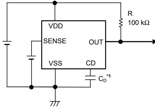
\*1. The delay capacitor ( $C_D$ ) should be connected directly to the CD pin and the VSS pin.
