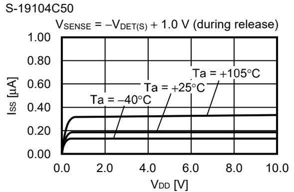
**6. Current consumption ( $I_{SS}$ ) vs. SENSE pin input voltage ( $V_{SENSE}$ )**
