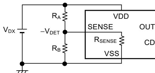
**Figure 24** Detection Voltage External Setting Circuit
