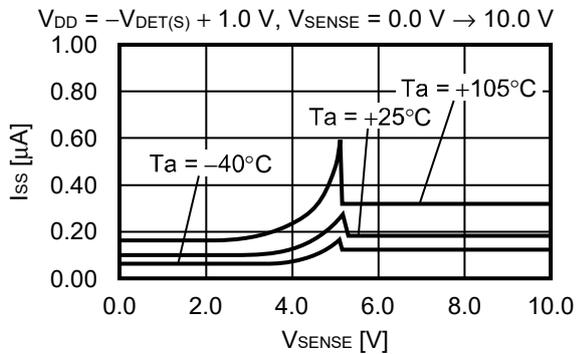
**7. Current consumption ( $I_{SS}$ ) vs. Temperature ( $T_a$ )**
