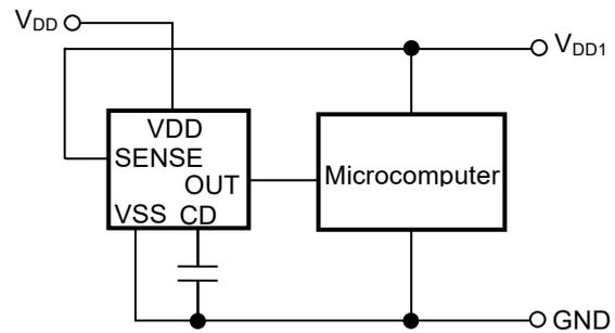
**Figure 37 Example of Reset Circuit
