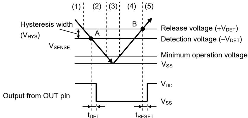
**Figure 23 Timing Chart of S-19104/19106 Series C Type**
