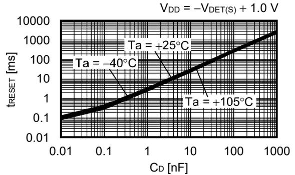
**16. Release delay time ( $t_{\text{RESET}}$ ) vs. Temperature ( $T_a$ )**
