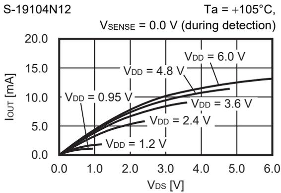
**9. Pch transistor output current ( $I_{OUT}$ ) –  $V_{DS}$**
