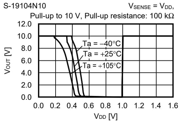
**13. Minimum operation voltage ( $V_{OUT}$ ) vs. SENSE pin input voltage ( $V_{SENSE}$ )**
