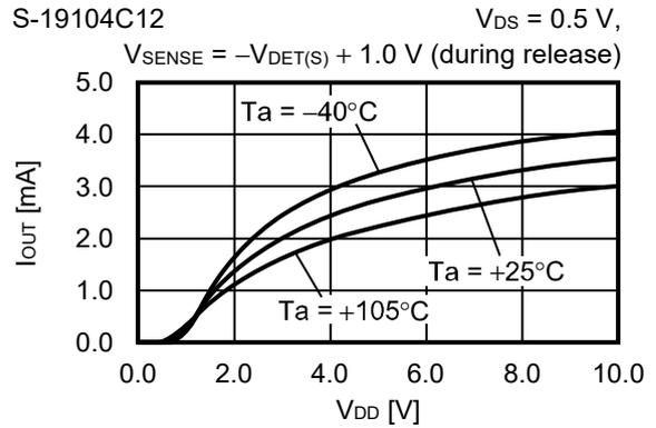
**12. Minimum operation voltage ( $V_{OUT}$ ) vs. Power supply voltage ( $V_{DD}$ )**
