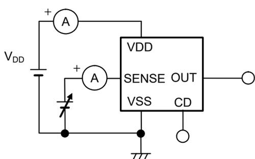
**Figure 7 Test Circuit 2**
