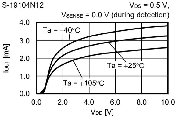
**11. Pch transistor output current ( $I_{OUT}$ ) vs. Power supply voltage ( $V_{DD}$ )**
