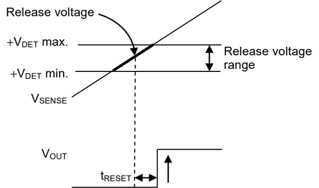
**Figure 15** Release Voltage
