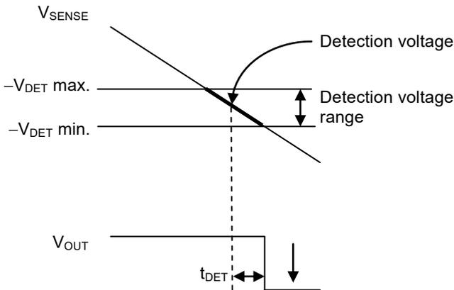
**Figure 14** Detection Voltage
