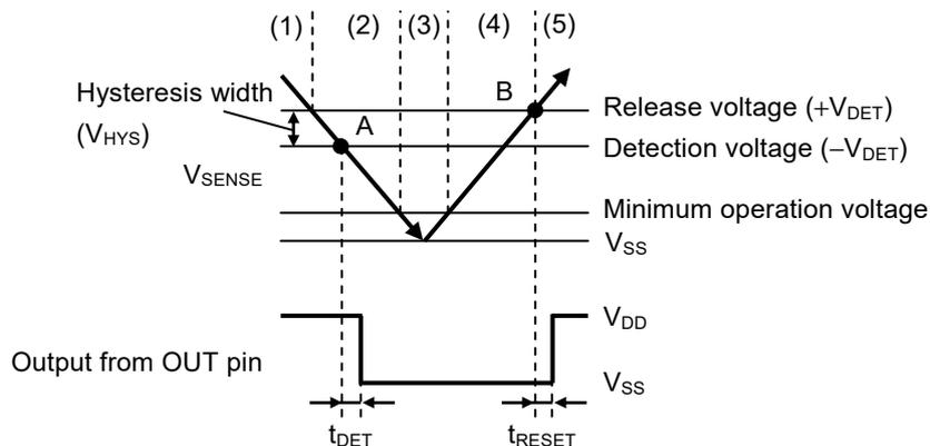
**Figure 21 Timing Chart of S-19104/19106 Series N Type**
