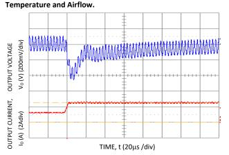
Figure 22. Transient Response to Dynamic Load Change from 50% to 100% at 28Vin, Cext - 1x10uF ceramic, CTune=150pF & RTune=220 $\Omega$
