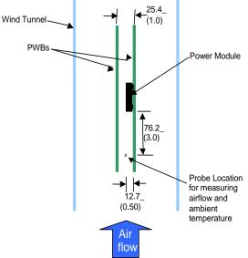
Figure 39. Thermal Test Setup.
