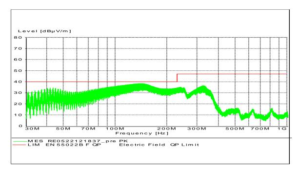
Fig 43 – EMI Plot of APXW005 on evaluation board with 24 V in @  $0.9 \, A$  in /  $5 \, Vdc$  @  $4 \, A$  out
