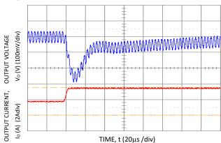
Figure 16. Transient Response to Dynamic Load Change from 50% to 100% at 28Vin, Cext - 3x10uF ceramic, CTune=470pF & RTune=150 $\Omega$
