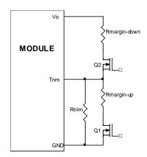
Figure 37. Circuit Configuration for margining Output voltage
