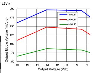
Figure 67. Output ripple with  $1x10\mu F$ ,  $2x10\mu F$  or  $4x10\mu F$  output ceramic capacitors (max load).
