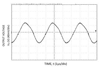
Figure 15. Typical output ripple and noise ( $V_{IN} = 28V$ ,  $I_0 = I_{0,max}$ ).
