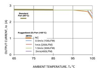
Figure 20. Derating Output Current versus Ambient
