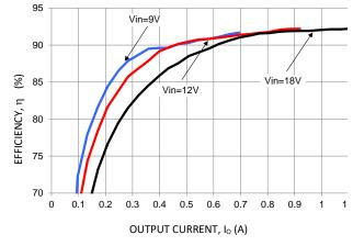
Figure 50. Converter Efficiency versus Output Current.
