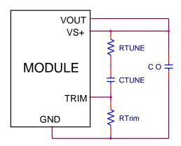
Figure. 38. Circuit diagram showing connection of  $R_{\text{TUME}}$  and  $C_{\text{TUNE}}$  to tune the control loop of the module.
