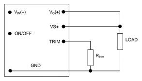
Figure 36. Circuit configuration for programming output voltage using an external resistor.
