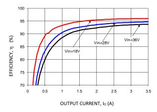
Figure 13. Converter Efficiency versus Output Current.
