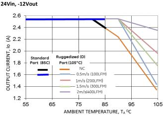
Figure 59. Derating Output Current versus Ambient Temperature and Airflow.
