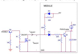
Figure 45. On/Off Level Shifting Circuit for the 5A ProLynx module for negative output applications.
