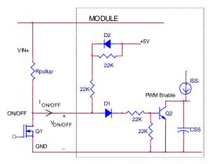
Figure 33. Circuit configuration for using negative On/Off logic.
