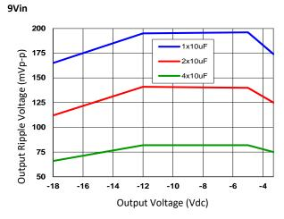
Figure 66. Output ripple with  $1x10\mu F$ ,  $2x10\mu F$  or  $4x10\mu F$  output ceramic capacitors (max load).
