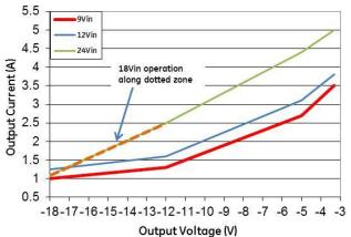
9Vdc -36Vdc input; 3Vdc to 18Vdc output; 5A to 2.5A Scaled output current 9Vdc -24Vdc input; -3.3Vdc to -18Vdc output; 5A to 0.7A Scaled output current
