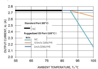
Figure 54. Derating Output Current versus Ambient Temperature and Airflow.
