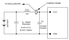
NOTE: Measure input reflected ripple current with a simulated source inductance ( $L_{\rm TST}$ ) of 1 $\mu$ H. Capacitor C<sub>S</sub> offsets possible battery impedance. Measure current as shown above.
