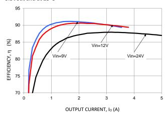
Figure 47. Converter Efficiency versus Output Current.
