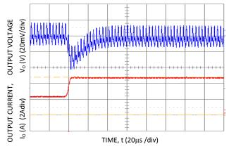
Figure 10. Transient Response to Dynamic Load Change from 50% to 100% at 28Vin, Cext - 10uF ceramic + 330uF polymer, CTune=10nF & RTune=150 $\Omega$
