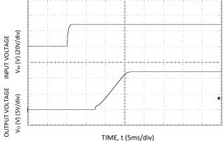
Figure 18. Typical Start-up Using Input Voltage ( $V_{IN} = 28V$ ,  $I_0 = I_{O,max}$ ).
