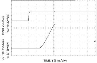
Figure 24. Typical Start-up Using Input Voltage ( $V_{IN} = 28V$ ,  $I_0 = I_{O,max}$ ).
