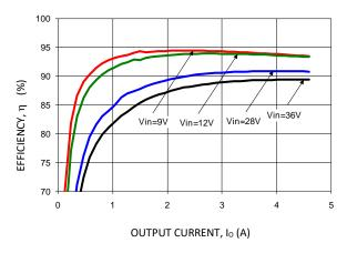
Figure 7. Converter Efficiency versus Output Current.
