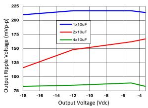
Figure 68. Output ripple with  $1x10\mu F$ ,  $2x10\mu F$  or  $4x10\mu F$  output ceramic capacitors (max load).
