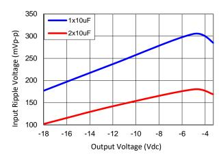
Figure 63. Input ripple voltage with 1x10  $\mu\text{F}$  or 2x10  $\mu\text{F}$  ceramic capacitors at the input (max load).
