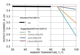
Figure 51. Derating Output Current versus Ambient Temperature and Airflow.
