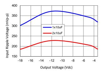
Figure 65. Input ripple voltage with 1x10  $\mu\text{F}$  or 2x10  $\mu\text{F}$  input ceramic capacitors (max load).
