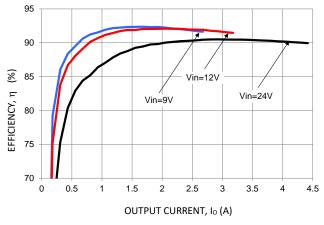
Figure 48. Converter Efficiency versus Output Current.
