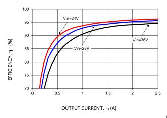
Figure 19. Converter Efficiency versus Output Current.
