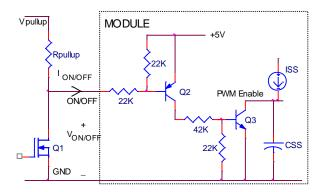
Figure 32. Circuit configuration for using positive On/Off logic.
