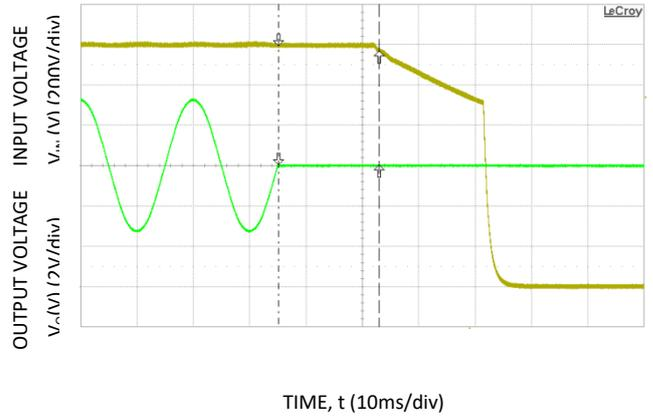
**Figure 8. Typical Hold-up waveforms ( $V_{IN} = 230V$ , 100% load).**
