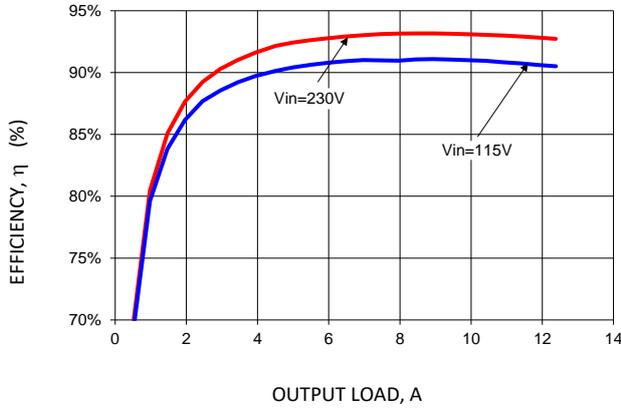
Figure 1. Power Supply Efficiency versus Output Current.
