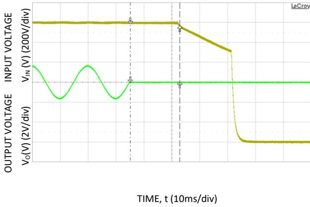
**Figure 7. Typical Hold-up waveforms ( $V_{IN} = 115V$ , 100% load).**
