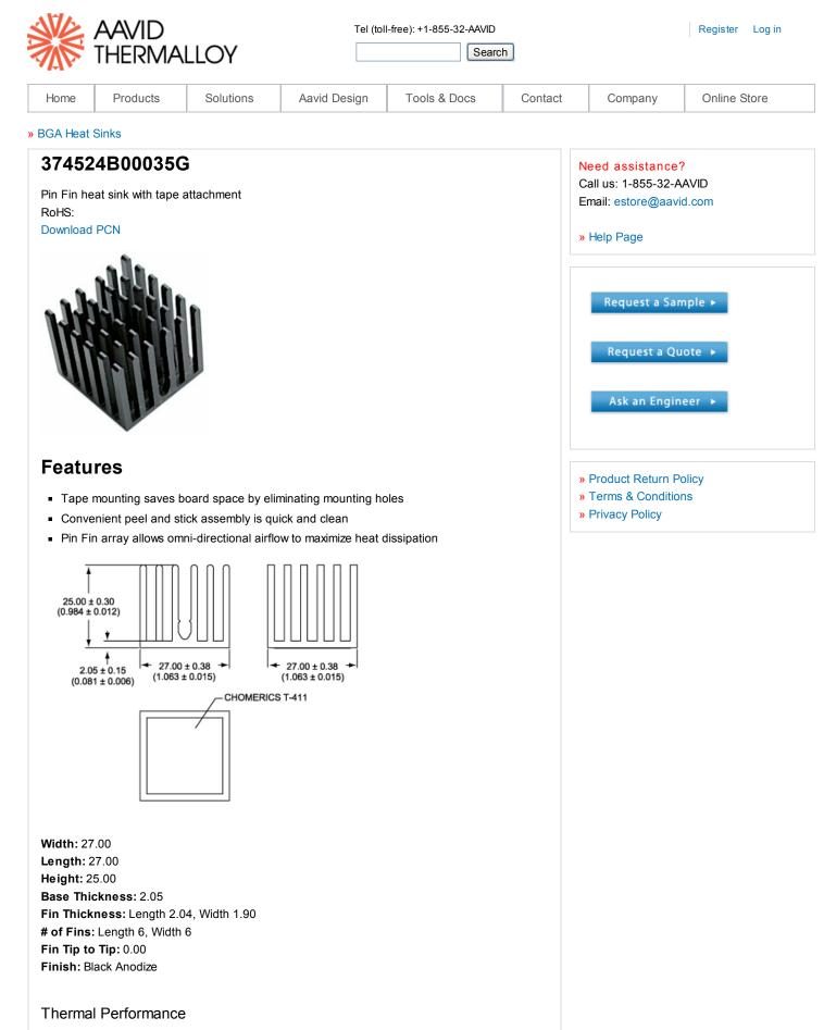
Natural Convection: 16.50 (based on a heatsink temperature rise of 75°C above ambient)
