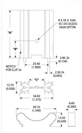
X Dim: 12.70 (0.500) | Y Dim: 0.79 (0.031) | Z Dim: 2.67 (0.105)
