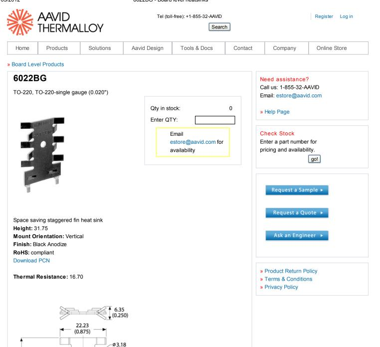
X Dim: 8.89 (0.350) | Y Dim: 0.50 (0.020) | Z Dim: 2.36 (0.093)
