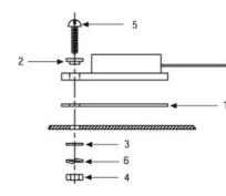
Note: Smooth side of flat washer should be placed against insulator when using the kit.
