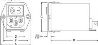
Mounting holes:  $\frac{.13}{3.3}$  Dia. (2) with .23 Dia. x 90° Counter sunk
