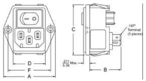
Mounting holes:  $\frac{.13}{3.3}$  Dia. (2) with .23 Dia. x 90° Counter sunk
